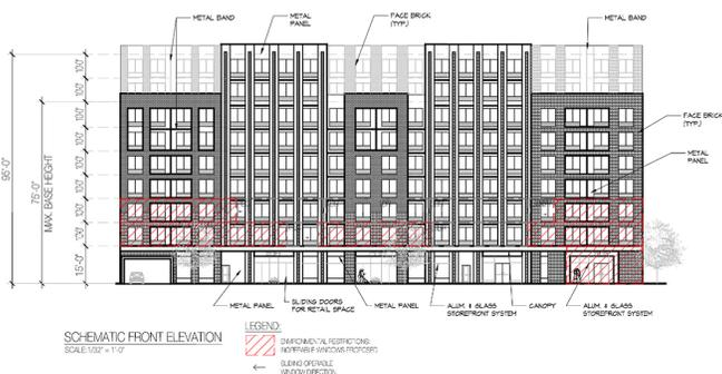
Elevation diagram illustrates proposed building components at 1340 Blondell Avenue (Aufgang Architects)
